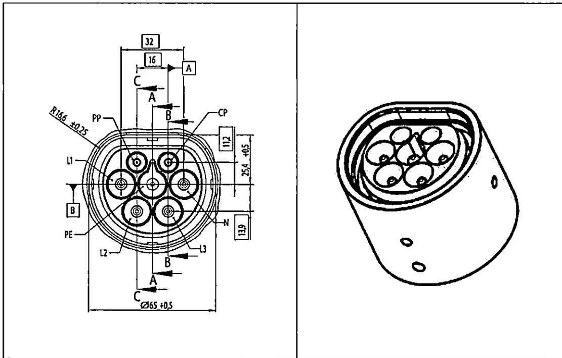
Gambar 4. *Inlet Kendaraan (Vehicle Inlet)*
