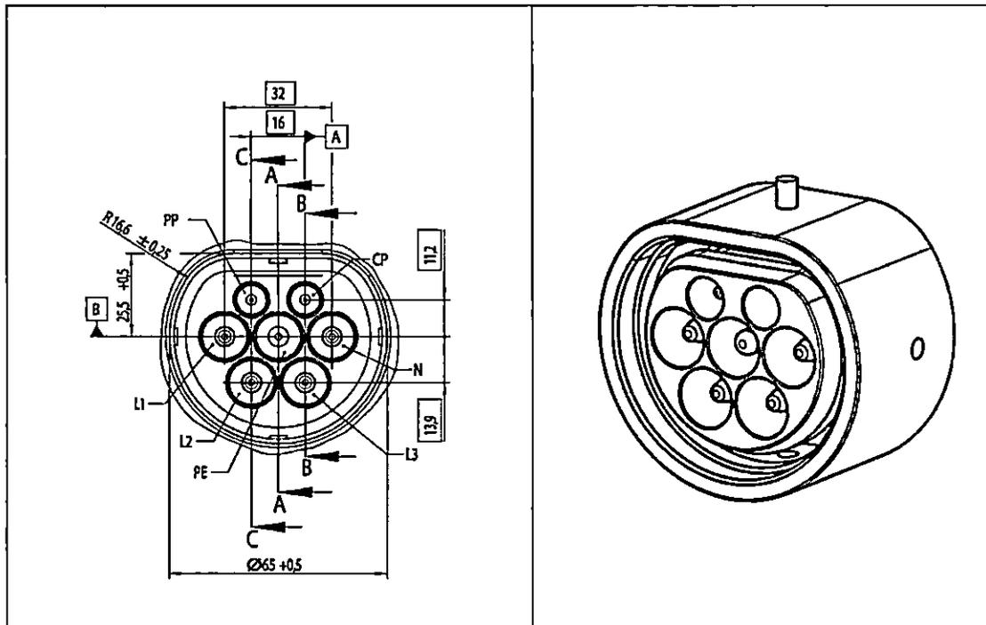
Gambar 6. *Inlet* Kendaraan (*Vehicle Inlet*)
