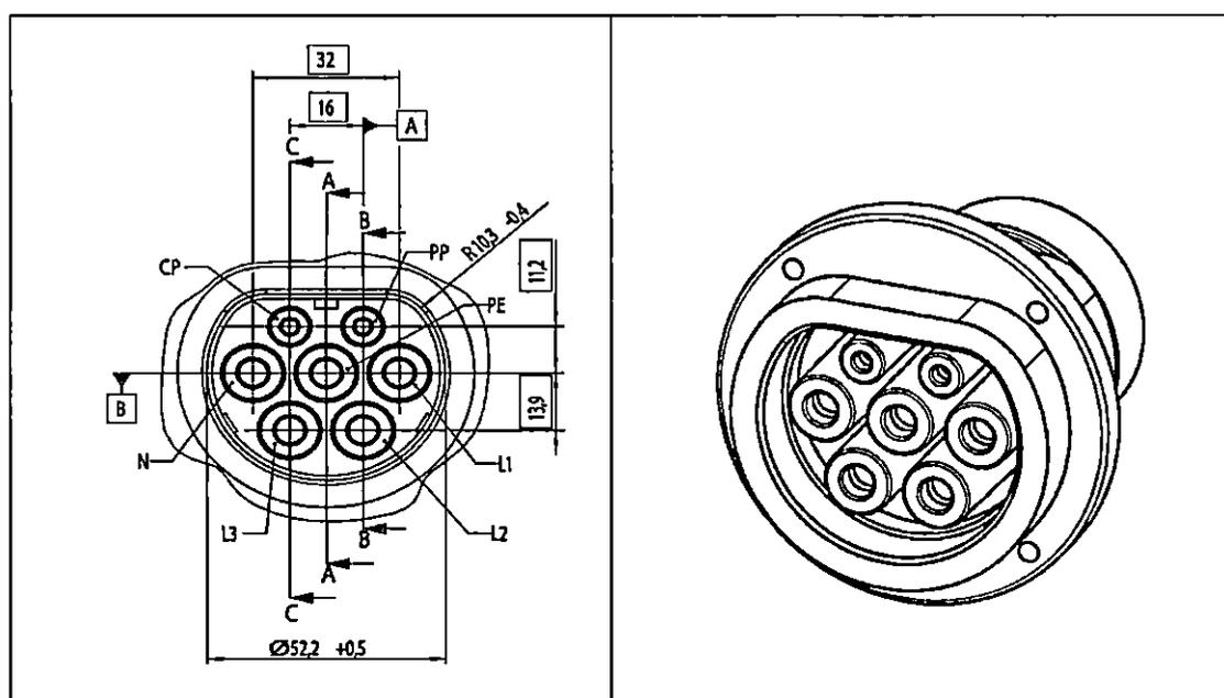
Gambar 1. Stop Kontak (*Socket Outlet*)
