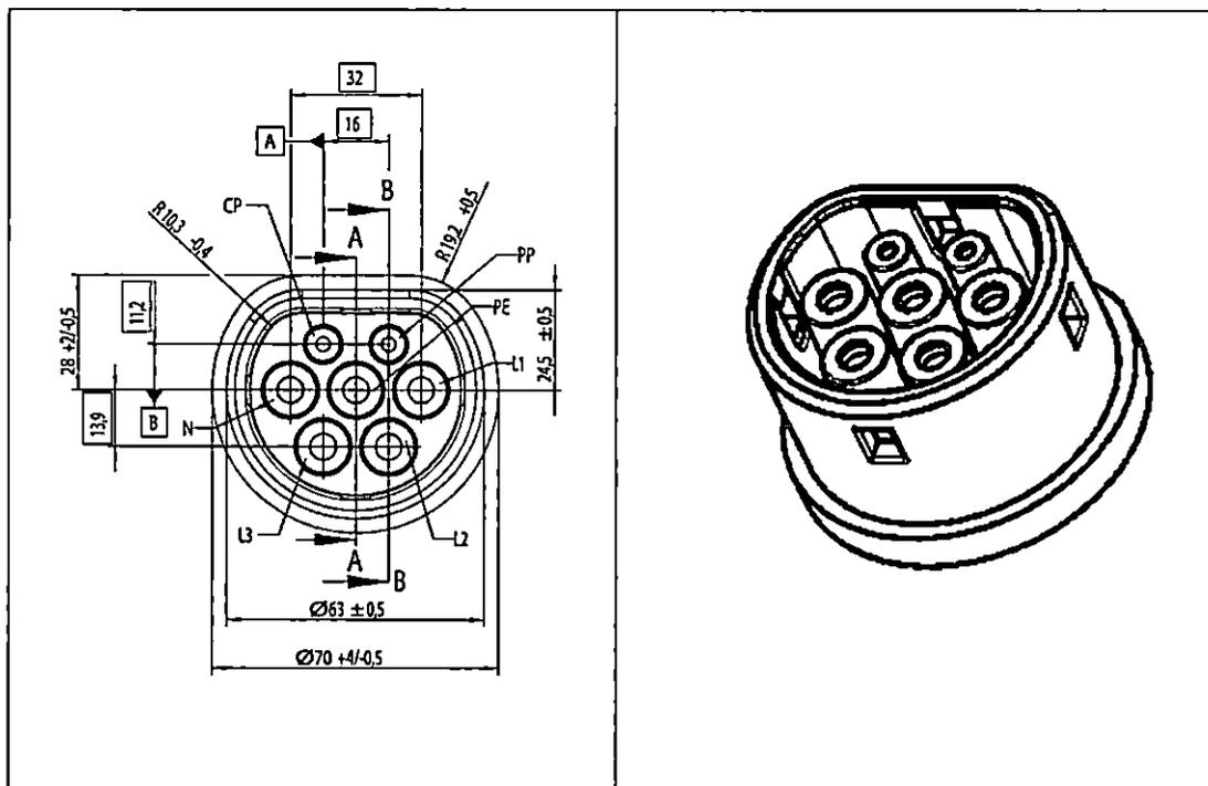
Gambar 5. *Konektor Kendaraan (Vehicle Connector)*
