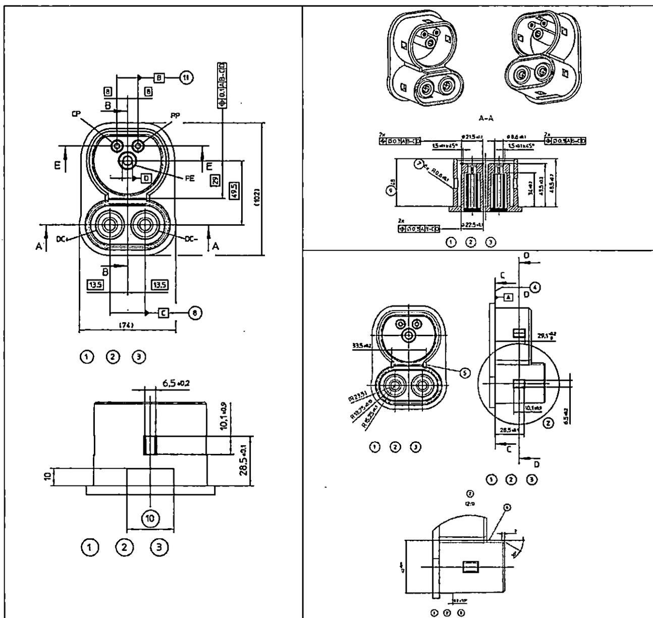
Gambar 12. Konektor Kendaraan Mode 4 (*Vehicle Connector Mode 4*)
